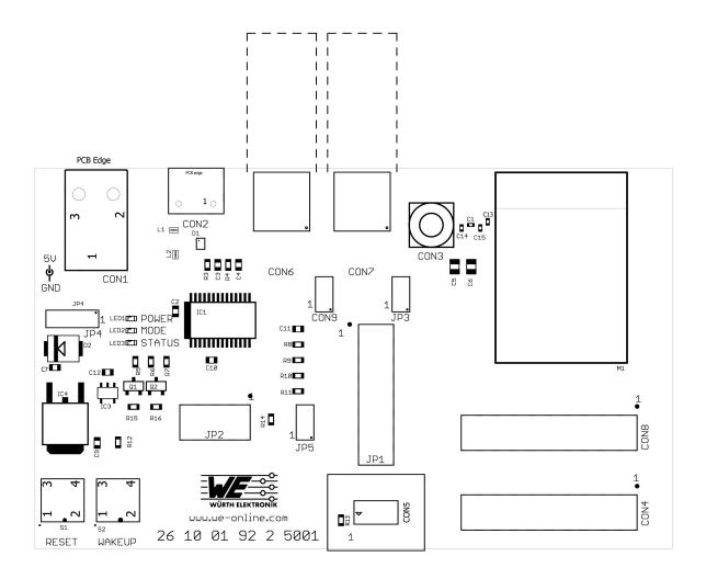
Figure 8: Assembly diagram
