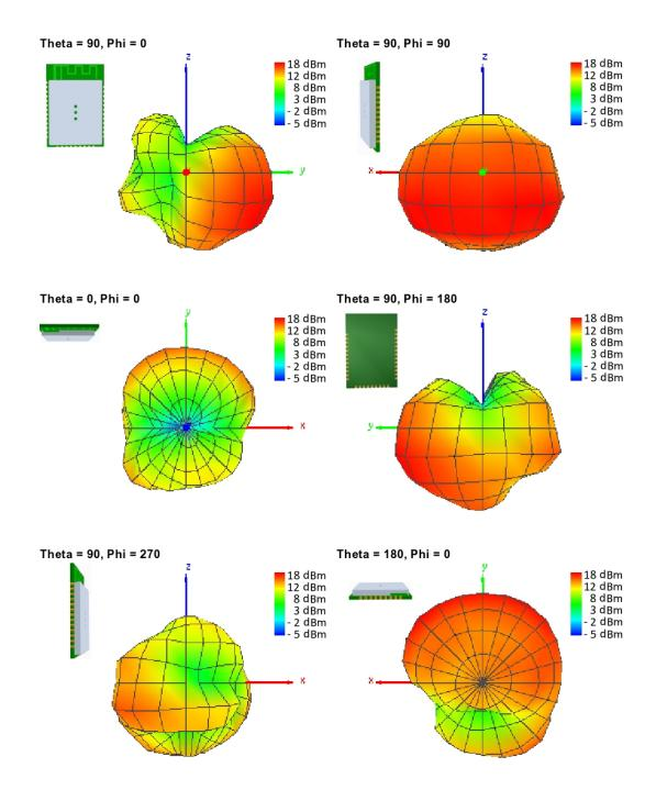
Figure 10: Antenna characteristic of the module with its integrated antenna measured on the official evaluation board
