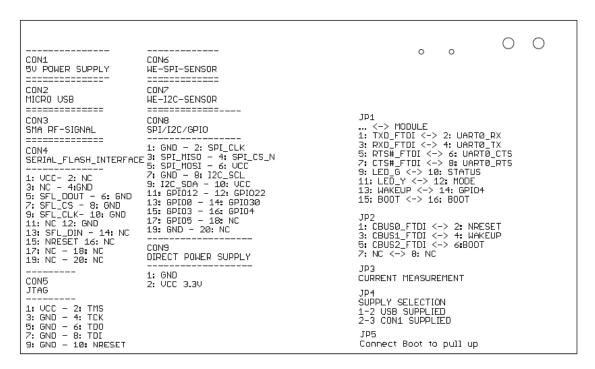
Figure 3: Quick Reference - Table of connectors and jumper
